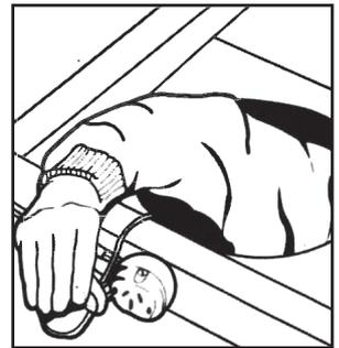
4. The Exhaust Fan is supplied with lead and 2 pin plug. Ensure that a power outlet is installed near the fan. (This outlet may be controlled by a standard switch or time delay switch.) Check power to the outlet is off. Plug the fan into this power outlet.
